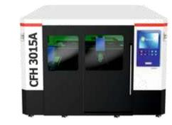
Fiber Laser Cutting Machine Close Type With Auto Pallet Changer
